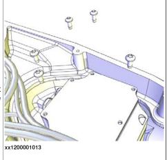
7 Secure the cable harness with cable straps to the heat protection plate.
