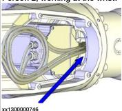
12 Remove the cable harness out of the arm Person 1, working at side hole: tube, at the back of the upper arm.
