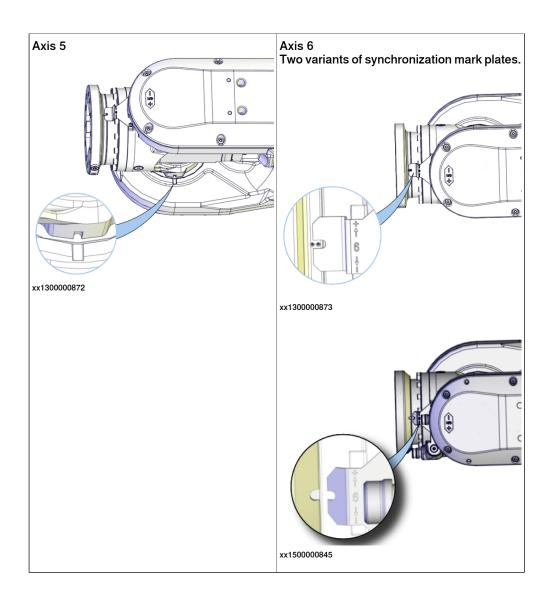
5.2.2 Calibration movement directions for all axes
