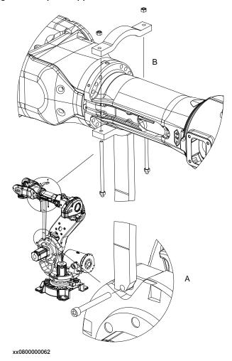
2.3.2 Securing the robot with a transport support *Continued*
