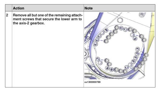
Removing and lifting away the lower and upper arms un-separated (Step 2)
