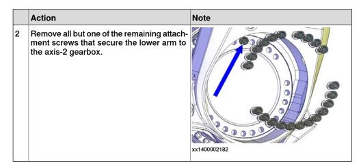
Removing and lifting away the lower and upper arms un-separated
